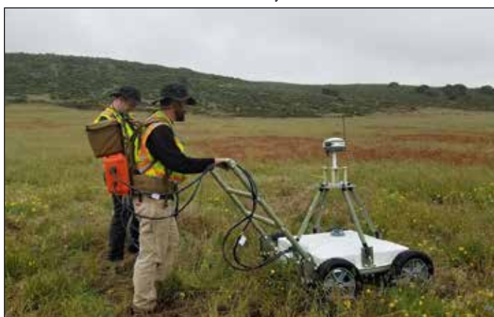
Technicians use electromagnetic metal detector at FUDS site.
